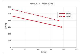
NOTE: Graph shows inlet pressure at a temperature of 68°F (tolerance ±10%)
