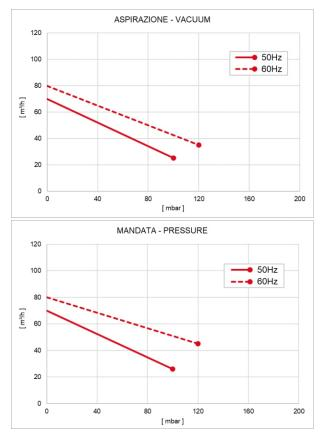
NOTE: Graph shows inlet pressure at a temperature of  $68^{\circ}F$  (tolerance ±10%)
