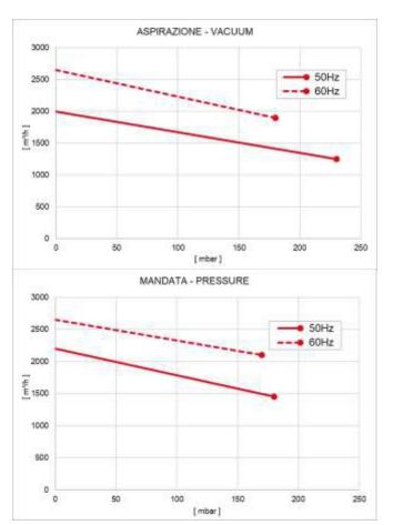
NOTE: Graph shows inlet pressure at a temperature of 68°F (tolerance  $\pm 10\%$ )
