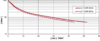
NOTE: Graph shows inlet pressure at a temperature of  $68^{\circ}F$  (tolerance ±10%)
